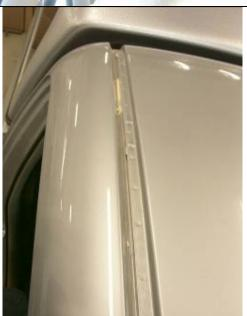
10.Unclip the exterior roof trim from both sides of the vehicle. Take care not to bend the trim, as it will be reused.
