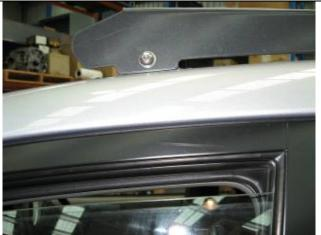
26. Fasten the mounting rails to the mounting blocks with M8 x 20mm button head screws, spring washers and flat washers and tighten.
