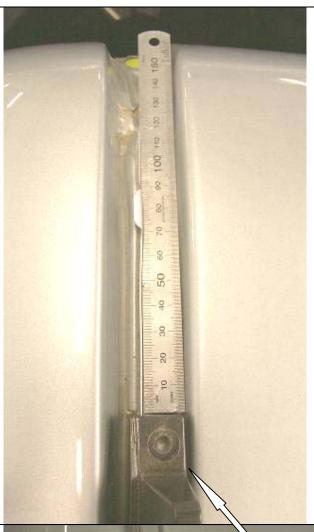
11. Position the rear mounting block as shown.
