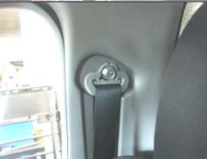
6. Remove the front and rear top seatbelt mounts.
