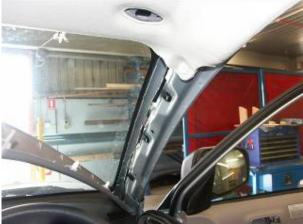
8. Remove the plastic trim from the front, middle and rear pillars on each side of the vehicle. They can simply be pulled away to be released from their mounting clips.
