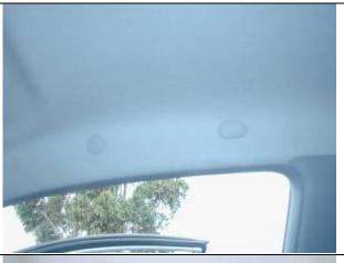
2. Remove the plugs on the driver's side of the vehicle, where there is no grab handle.
