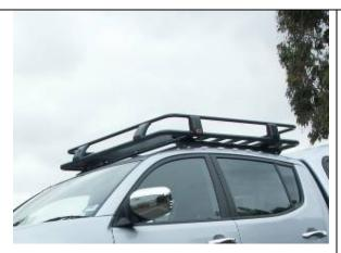
27. With the assistance of another person, lift the roof rack onto the vehicle and position evenly.
