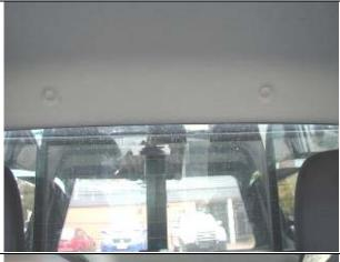
5. Remove the rear plugs holding the roof liner.
