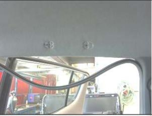
7. Pull down the door seals so the interior trim can be removed.
